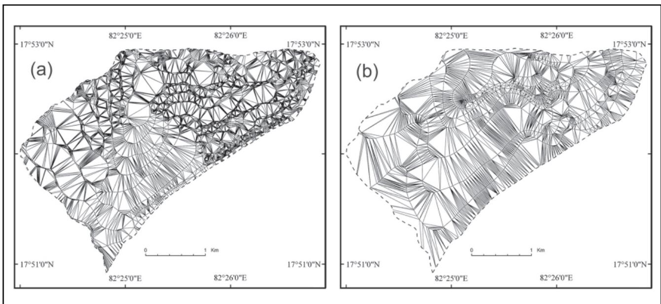
**Figure 4.** Triangulated Irregular Network (TIN) surfaces representing (a) surface configuration, and (b) bedrock configuration of the study area. These maps show the slope, aspect and elevations of the respective surfaces.
