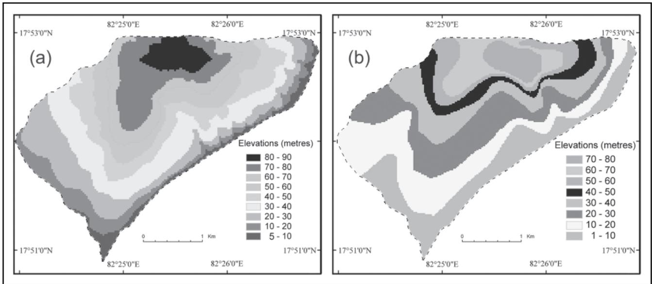
**Figure 5.** GRID maps of (a) surface configuration, and (b) bedrock configuration of the study area. The maps are composed of raster cells of 20m-by-20m area; hence the boundaries between various elevation ranges are not smooth.
