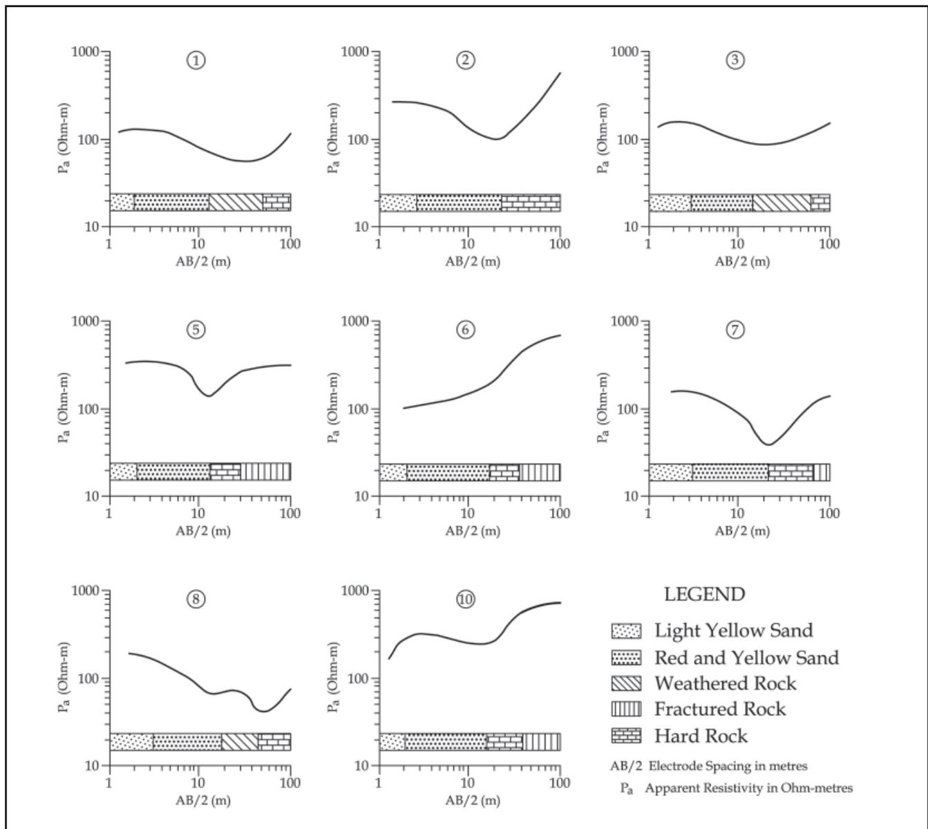
**Figure 2.** Sample resistivity curves showing the various subsurface layers in the study area. The locations of these eight curves are shown with encircled points and bold numbers in Figure 3a.
