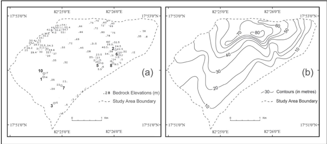
**Figure 3.** The study area showing (a) the bedrock elevations estimated at 100 locations based on geo-electrical resistivity surveys from which contours were interpolated representing (b) the bedrock configuration in the area. The encircled points with bold numbers in the left panel indicate the location of the sample resistivity curves shown in Figure 2.
